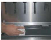
Step 2 Remove rack. Wipe down inside/outside of the drip pan with a clean cloth towel and Kay-5® or chlorine-based sanitizer solution.
