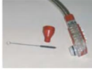
Follow steps 1 & 2 of Cleaning the Dispensing Valves, then remove nozzle & clean nozzle/diffuser with a dedicated brush and sanitizer solution. Let them air dry and reinstall nozzle.
