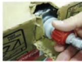
Step 5 Shake BIB connector a couple of times and reconnect syrup lines to correct Bag-in-Boxes.
