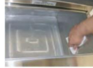
Step 3 Clean all interior sides with a clean cloth towel and Kay-5® or chlorine-based sanitizer solution. Wipe dry.
